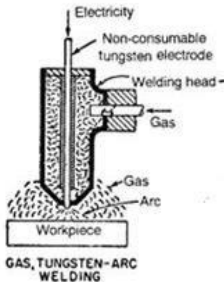
Figure 3.13 Tungsten inert gas arc welding
