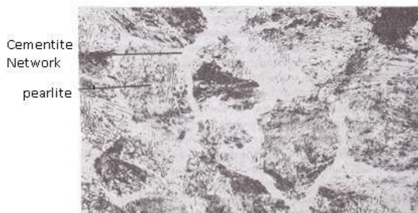
Fig.5.11 - Photomicrographs of (a) 1 percent carbon steel, slow – cooled, 500X; (b) 1.2 percent carbon steel, slow – cooled, 300X.
